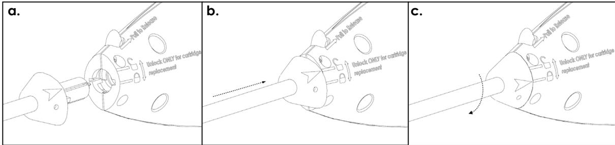
***Figure 2- Cartridge loading process***
