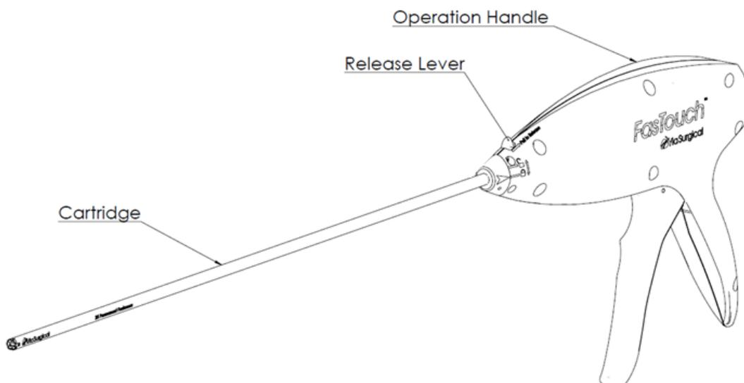
**Figure 1- Schematic view of the FastTouch™ device**
