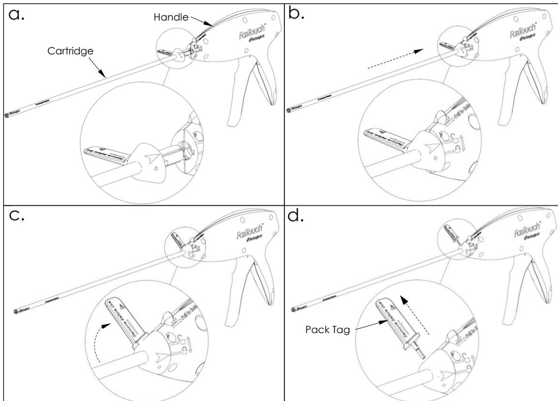
**Figure 2- Cartridge loading process**
